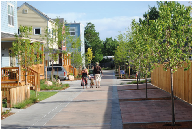
Example of calmed one-way street incorporating footway, carriageway and limited off-street parking
