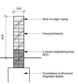
Brickwork Boundary Wall - Type W1 1:20 - Typical Section.
